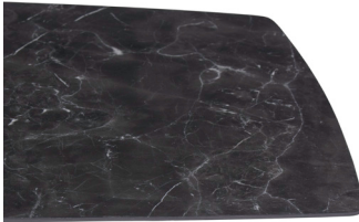
Ceramic marble th. 6mm reinforced by MDF E1 th. 17mm shaped bevelled at 25°. Curved 4 edges.
